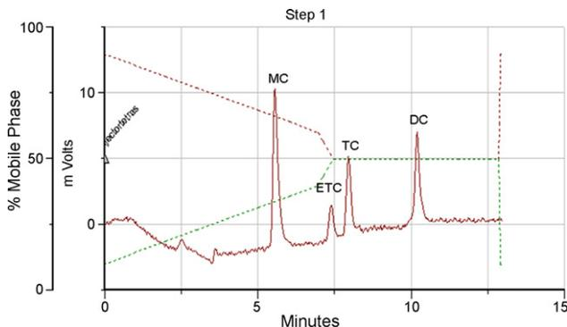
Fig. 2. HPLC–FD chromatogram of the standard solution of MC, ETC, TC and DC at 0.1, 0.05, 0.25 and 0.5  $\mu\text{g L}^{-1}$ , respectively. Mean retention times were for MC, ETC, TC and DC 5.89, 7.63, 8.25 and 10.51 min, respectively.
