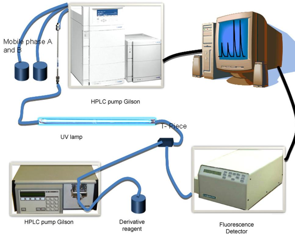
Fig. 1. Scheme of the HPLC-PIF method.
