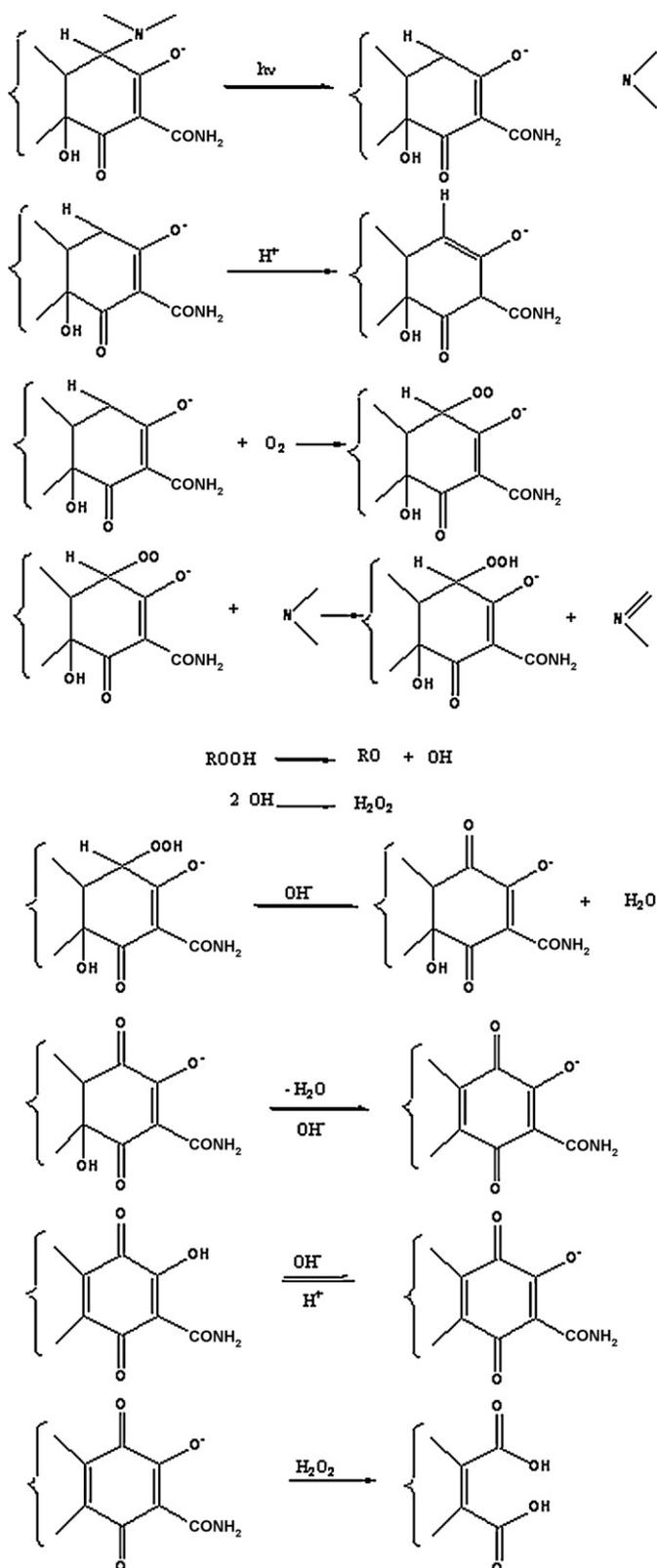
Fig. 4. Photodegradation pathway for the tetracyclines [21].
